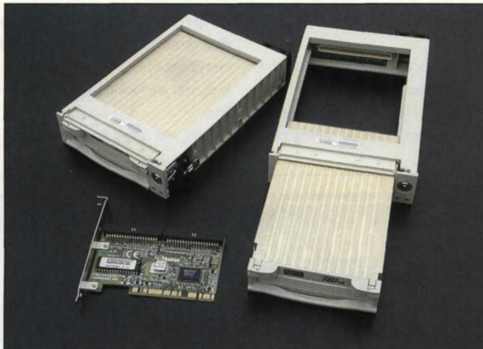
A removable drive bay is used to move a data drive quickly from one computer to another. The drive can be controlled from an IDE motherboard cable, or as part of a RAID system.
